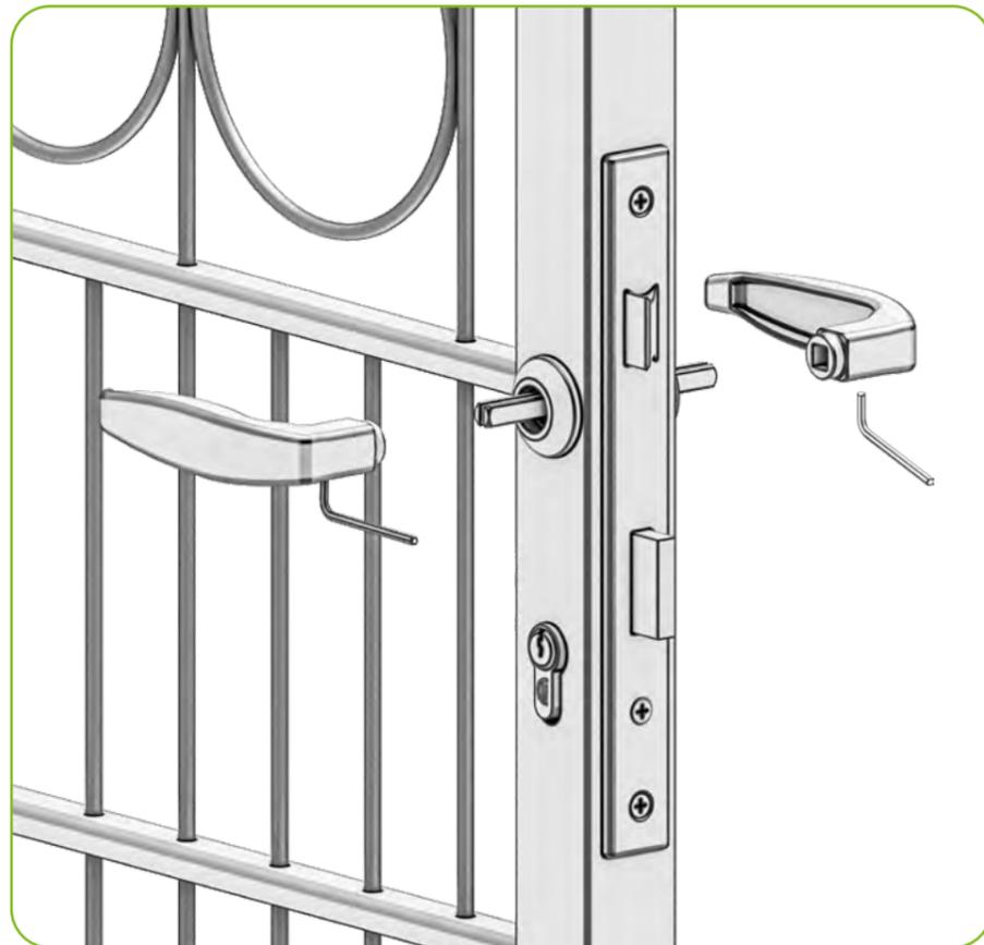
Insert the doorhandle pin through the lock and out through the other side. Slide the doorhandles on the pin on both sides and tighten them with the Allen key provided.
