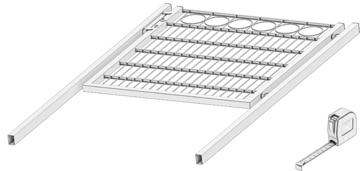
Lay out the gate parts on a soft surface and measure them. Determine the direction of rotation and position of the gate before placing the posts.
