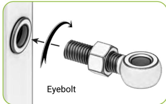
Pre-adjust the hinges to ease assembly later. Tighten the nut on the eyebolt and then tighten the eyebolt into the gate leaf. Do not tighten the nut against the gate leaf yet. Turn the eyebolt in the same number of turns on both hinges.
