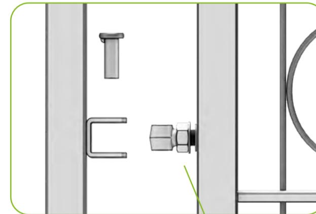
Tighten the nut on the eyebolt well so that the gate leaf is firmly attached to the eyebolt. Then hang the gate leaf in position.
