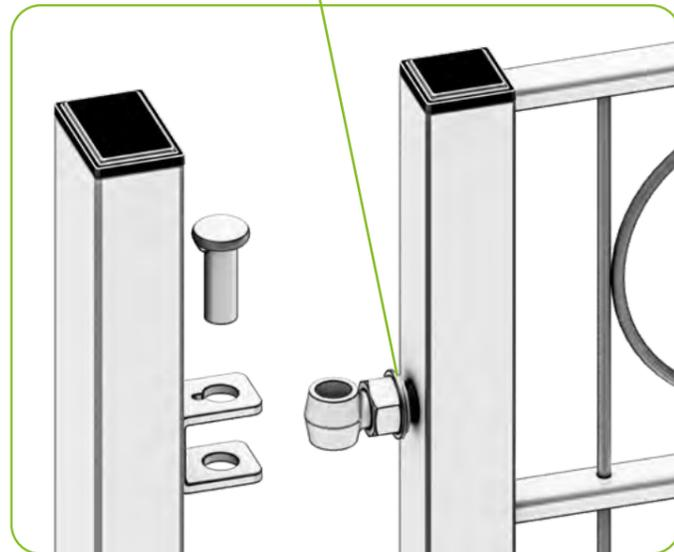
If you have too little or too much space between the posts than you had in mind, you can adjust the position of the eyebolt in the hinge plate by adjusting the position of the nuts on the eyebolt.
